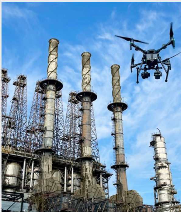
Photo: Unmanned aerial systems are used in Chevron's facilities to minimize personnel exposure and reduce inspection costs.
